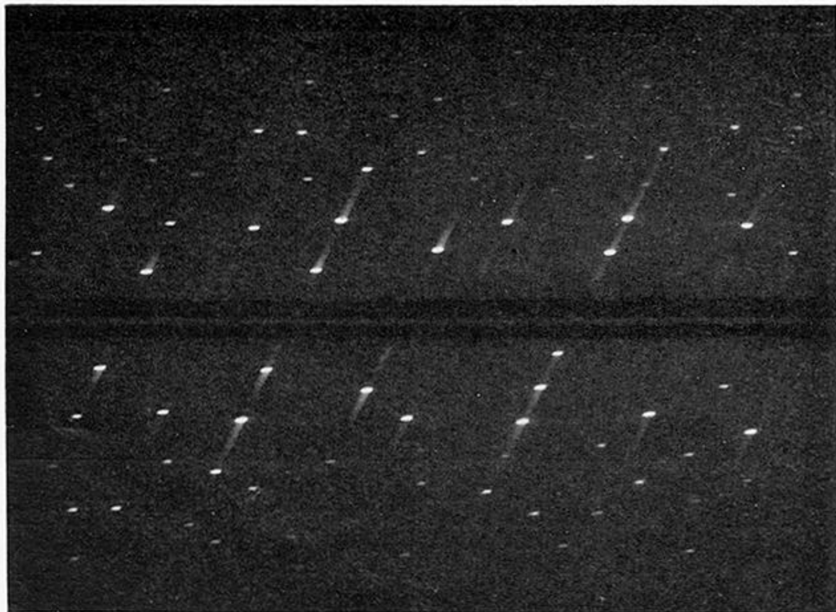
FIGURE 15. (a) Fresh p.o.a.: h0l Weissenberg photograph, \text{CuK}\alpha\beta . Good crystal. (b) h1l of another p.o.a. crystal, photograph strongly exposed.
